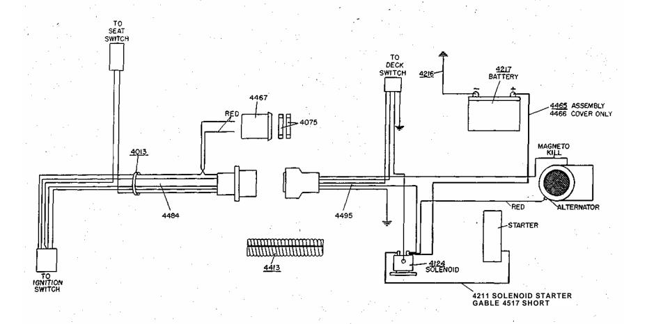
BODY WIRING LOOM - 4484 REAR WIRING LOOM-4495 WIRING KIT (308-311)-8669 (SEE ASSEMBLY BREAKDOWN)
